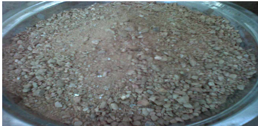
Fine aggregate having fineness modulus 3.19
