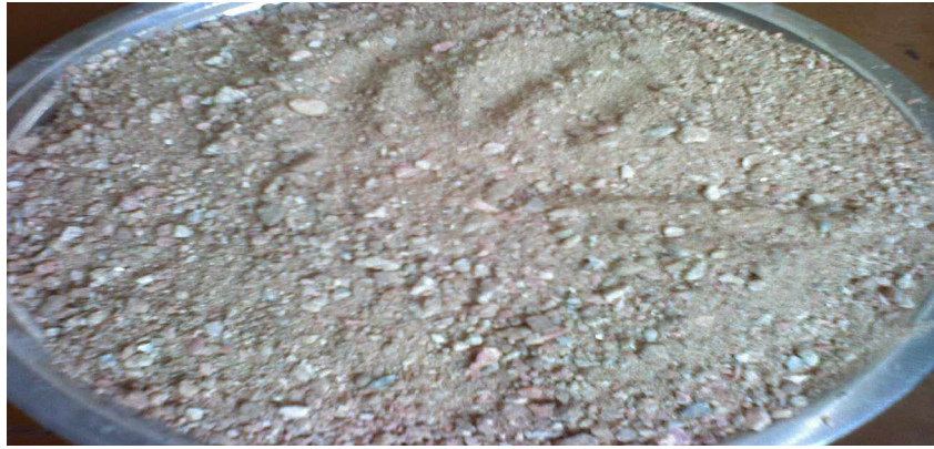
Fine aggregate having fineness modulus 2.92
