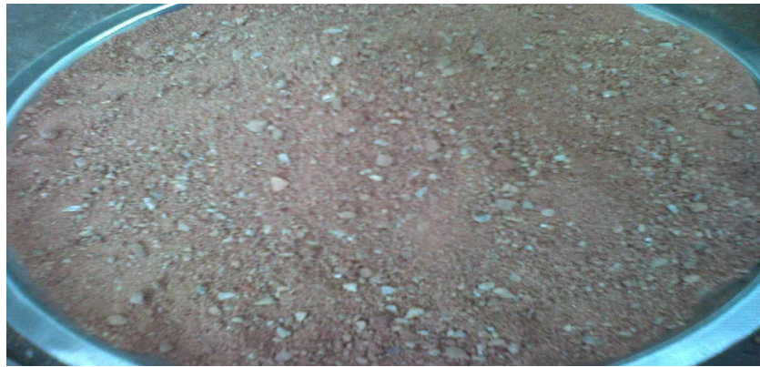
Fine aggregate having fineness modulus 2.1
