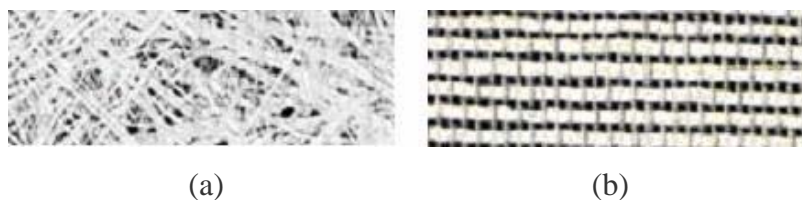
Figure 2 Illustration showing the difference between (a) Randomly oriented fibers and (b) Unidirectional woven fabric
