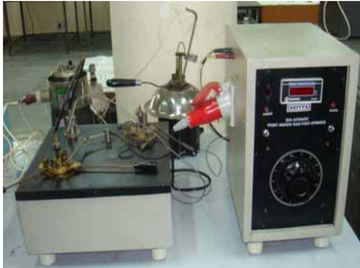
Plate 4.3: Pensky Marten Flash Point Apparatus
