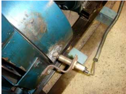
Plate 3.14: Engine Speed Measurement
