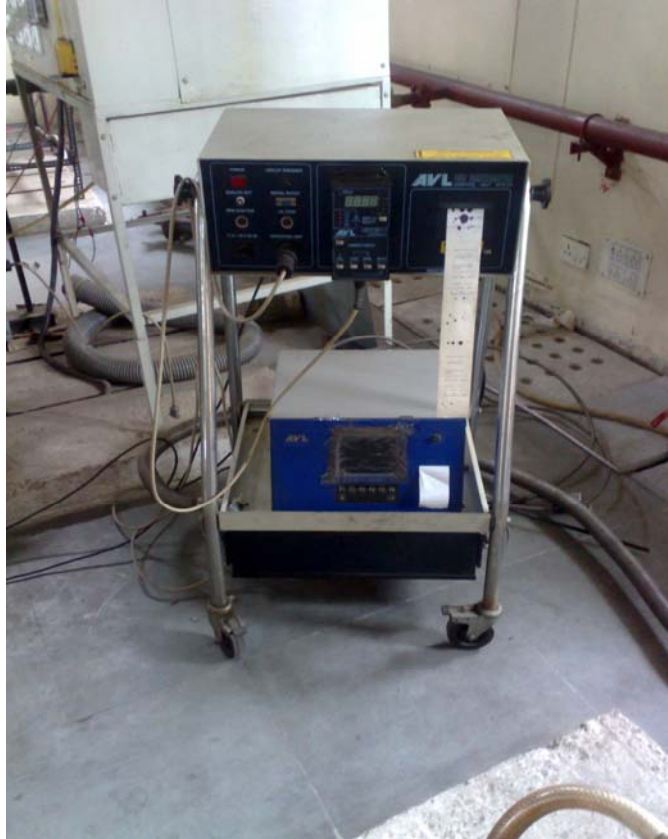
Plate 3.9: Smoke Meter and Di Gas Analyzer
