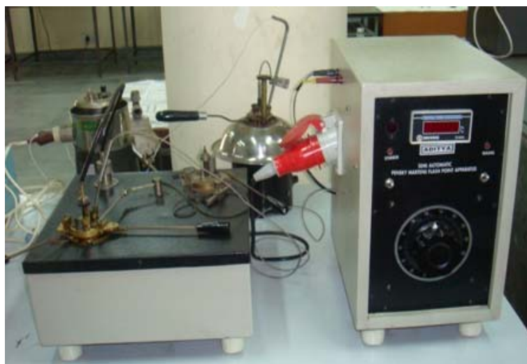
Plate 3.15: Pensky Marten Flash Point Apparatus
