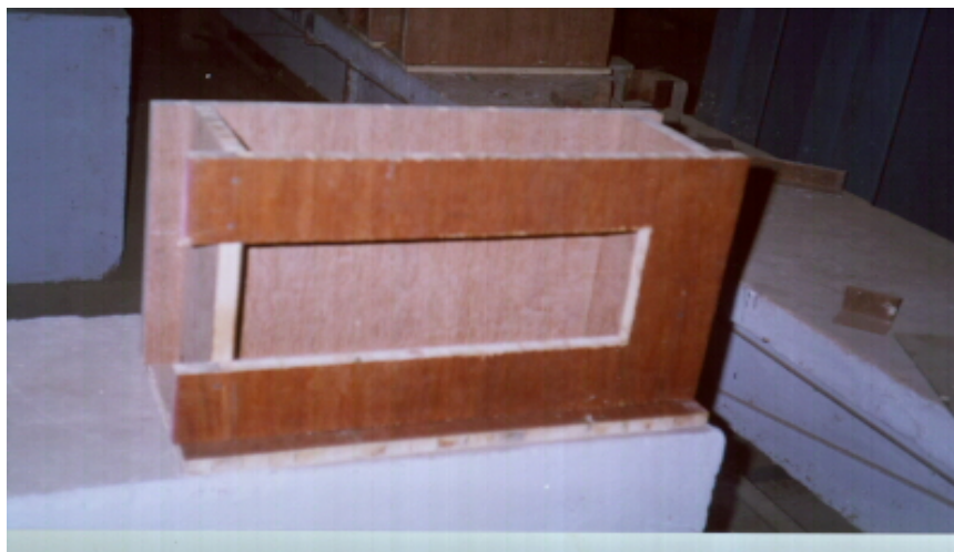
Fig. 16. Standard mould for composite push-out specimen.
