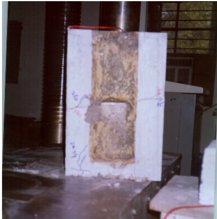
Fig. 36. Concrete slab of specimen IV after testing
