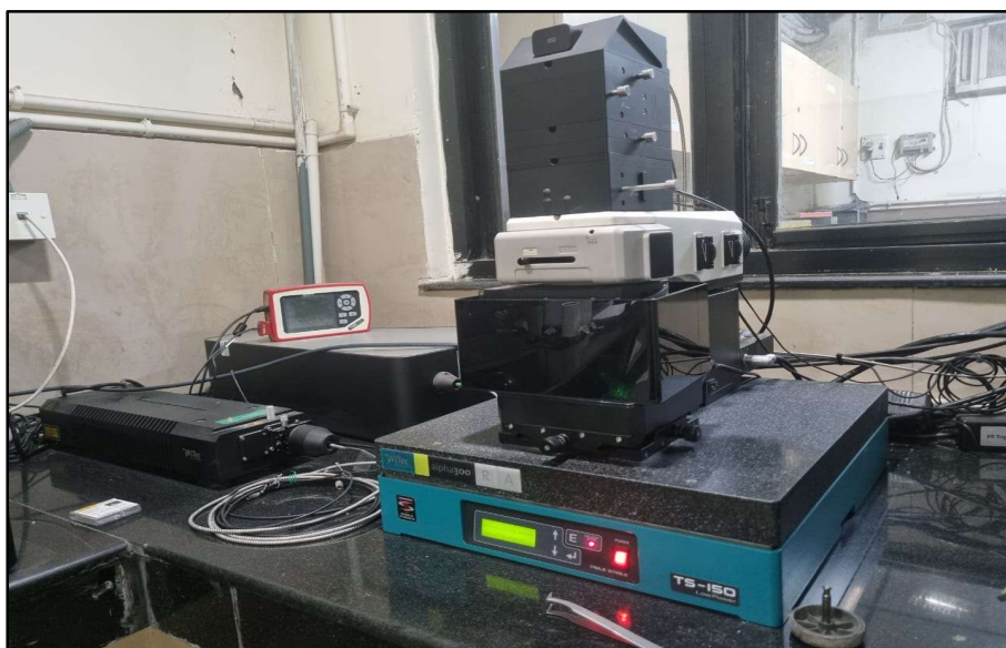
Figure 2.16: Picture of Witec Raman spectrometer
