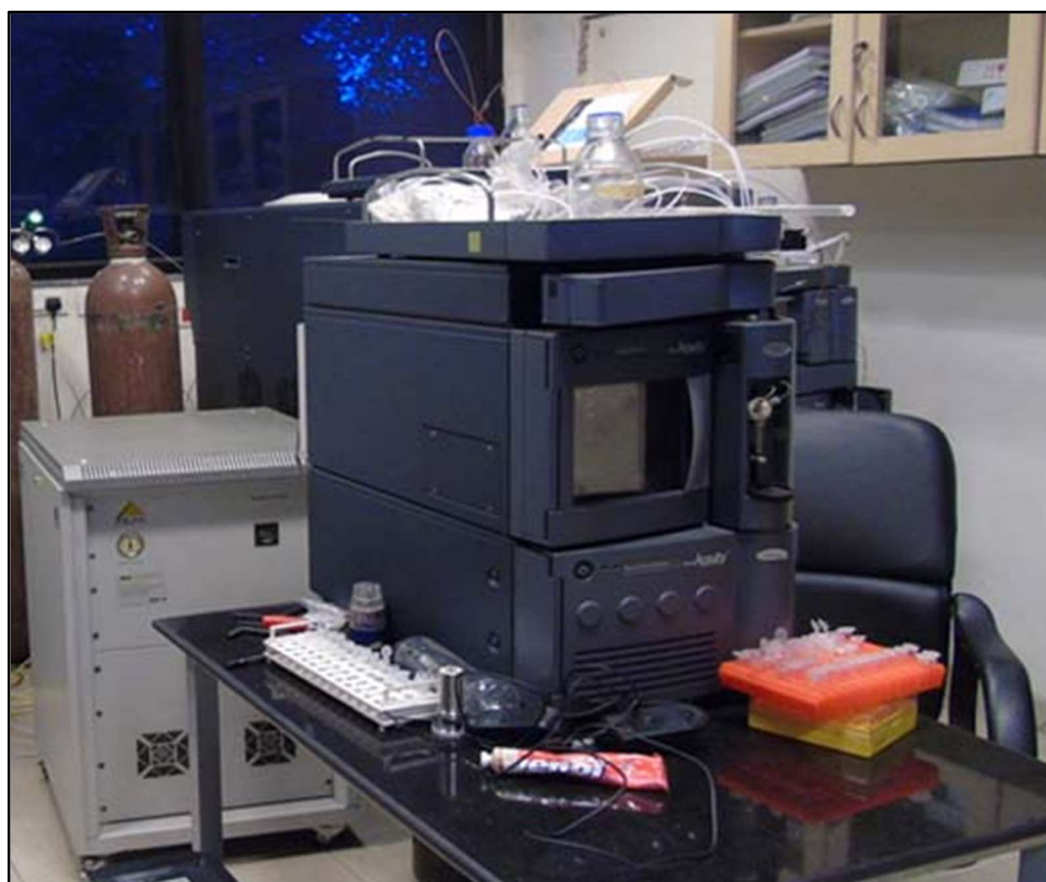
Figure 2.22: Picture of Waters SYNAPT G2 with 2D nano ACQUITY System
