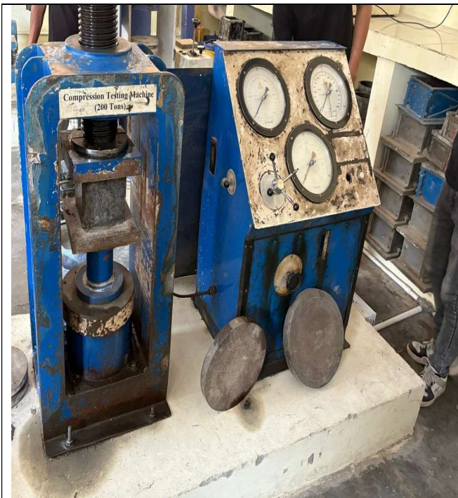
(e) Compressive strength testing
