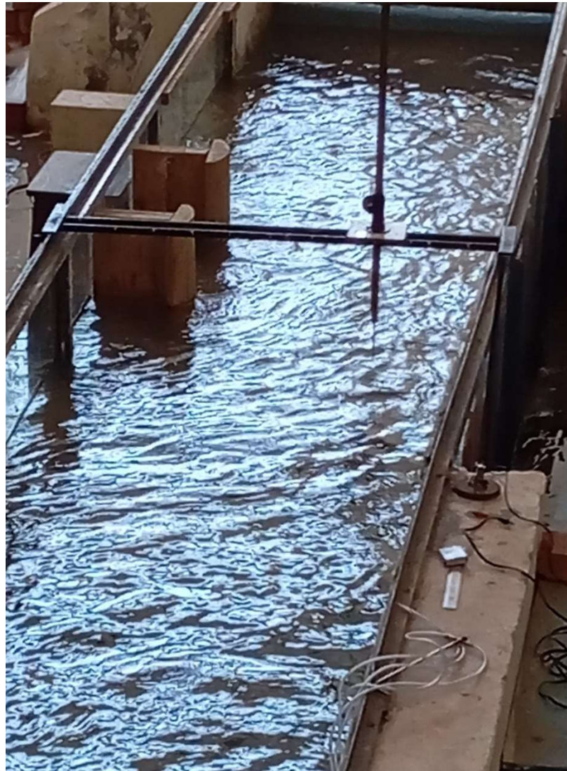
Figure 4.21: Experimental placing of two curved T-shape spur dikes in the working section of the flume
