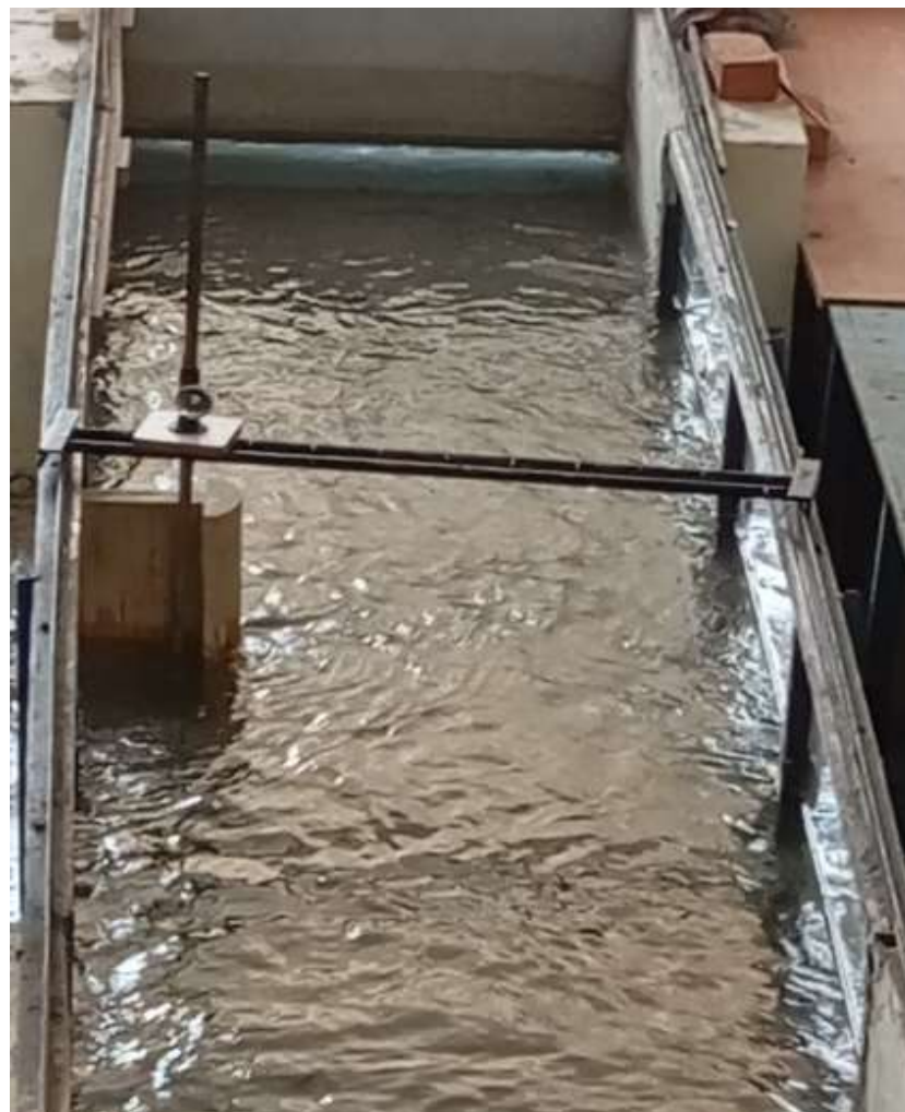
Figure 4.1: Experimental plan of masonry flume with curved T-shape spur dikes
