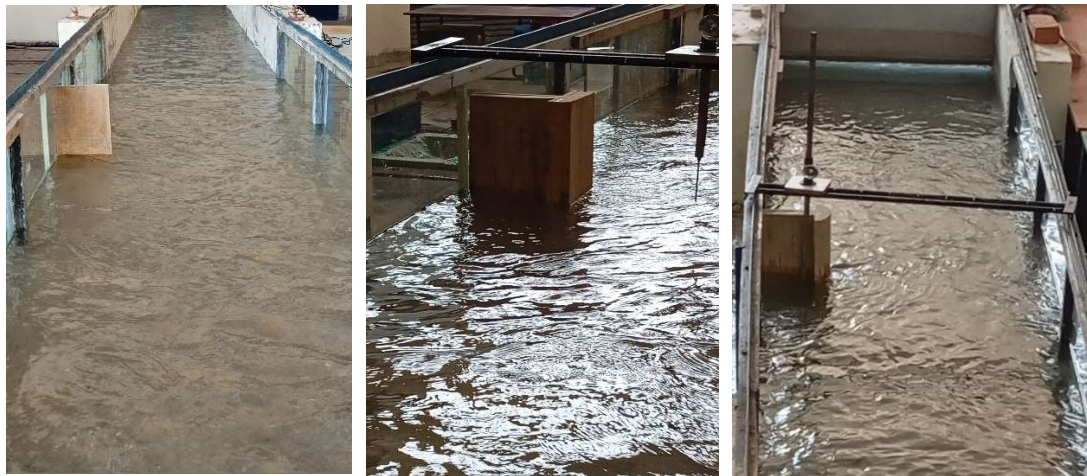
Figure 4.29: Placement of I-, T-, and curved T-shape spur dikes in the working section of the flume
