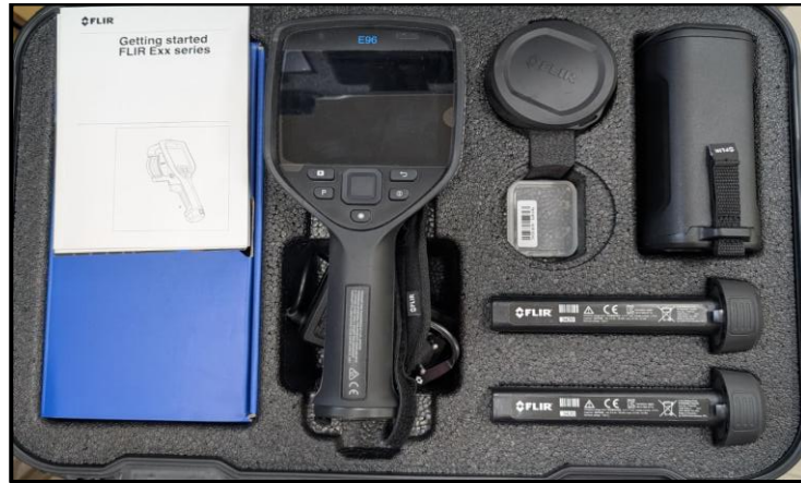
Figure 2.16: FLIR E96 infrared thermographic camera
