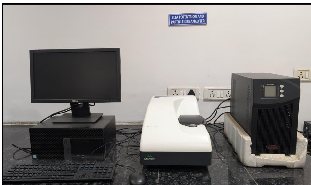
Figure 2.13: Malvern zetasizer nano ZS
