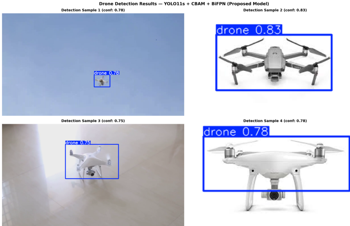
Figure 4.4: Qualitative drone detection results across four surveillance scenarios
