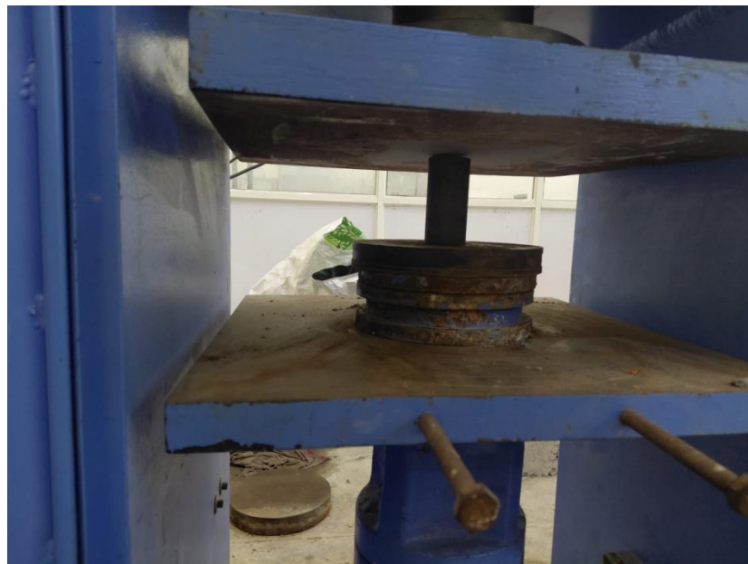
Figure 4.12: Rock specimen placed in the compression testing machine for UCS testing.
