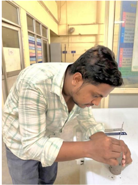
Figure 4.9: Measuring of Crack width with bore gauge .
