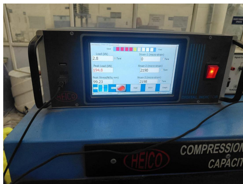
Figure 4.14: UCS test result displayed on the digital control panel.
