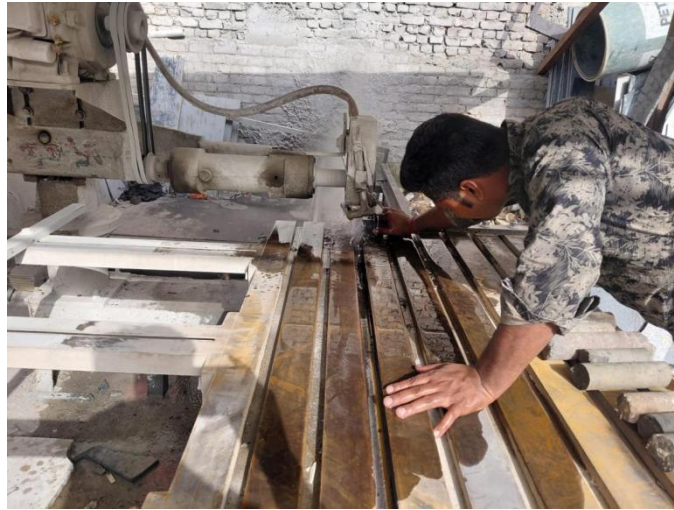
Figure 4.3: Sample preparation of rock core specimens using a core cutting machine.
