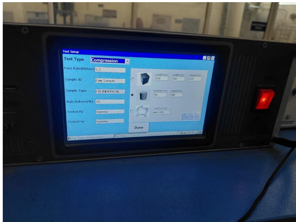
Figure 4.13: UCS test setup on the digital control panel showing sample type, dimensions and pace rate.
