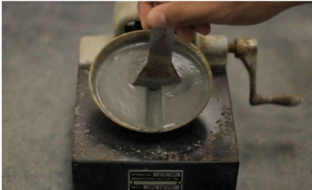
Figure 3.5: Determination of liquid limit using the Casagrande liquid limit apparatus, showing the liquid limit cup and groove formation
