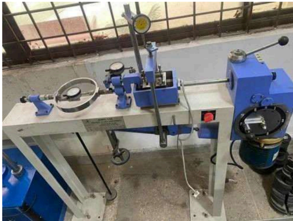
Figure 3.7: Direct shear testing apparatus for shear-strength evaluation
