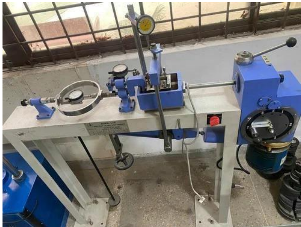
Figure 3.7: Direct shear testing apparatus for shear-strength evaluation
