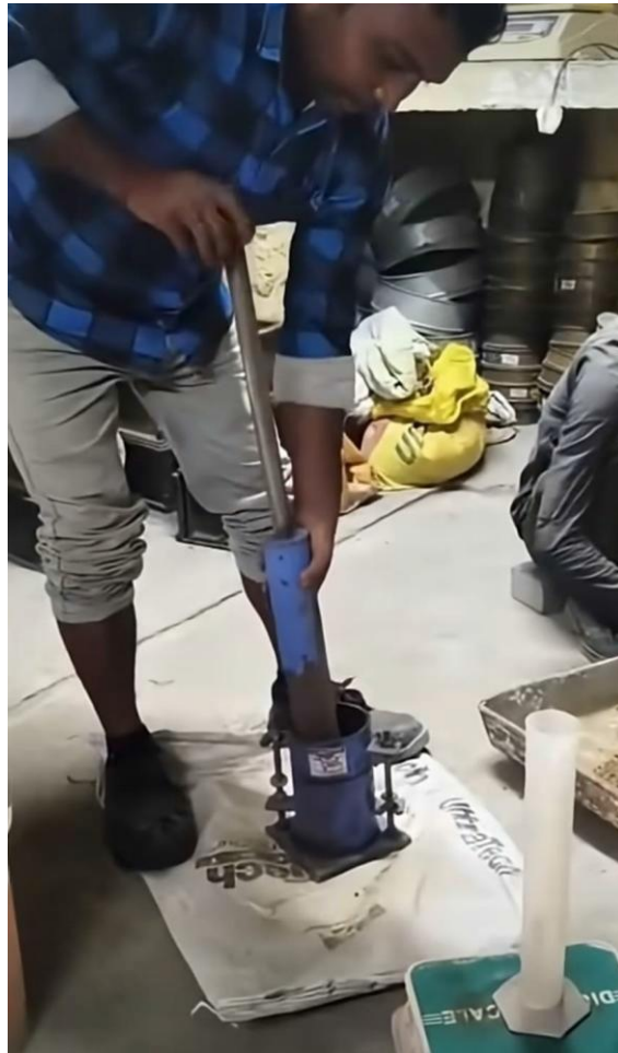
Figure 3.6: Standard Proctor compaction test setup
