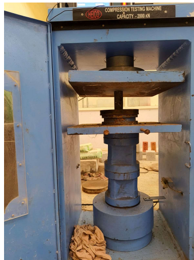
Figure 3.4: Uniaxial Compressive Strength (UCS) Test Conducted on the Cylindrical Rock Specimen
