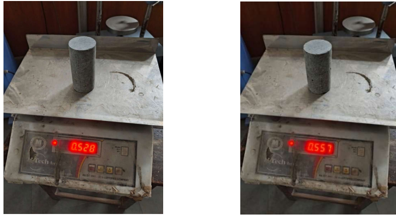
Figure 4.3 Weight of rock Sample (a) Dry (b) Saturated
