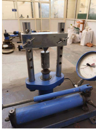
Figure 3.3: Experimental Setup for the Axial Point Load Strength Index ( I_{ss0} ) Test
