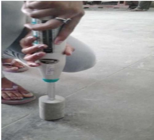
Figure 4.4: Schmidt Hammer Rebound Test
