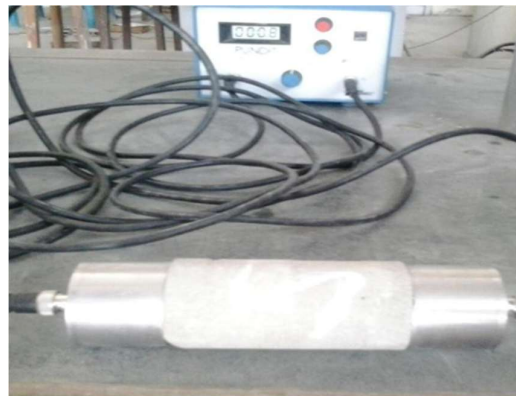
Figure 4.5: Ultrasonic Pulse Velocity (P-wave Velocity) Test
