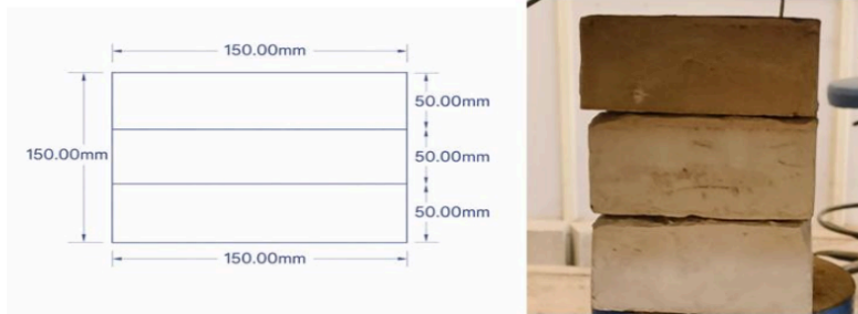
Figure 3. 4 Arrangement of blocks with zero degree orientation
