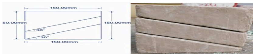
Figure 3.6 Arrangement of blocks with 30 degree orientation
