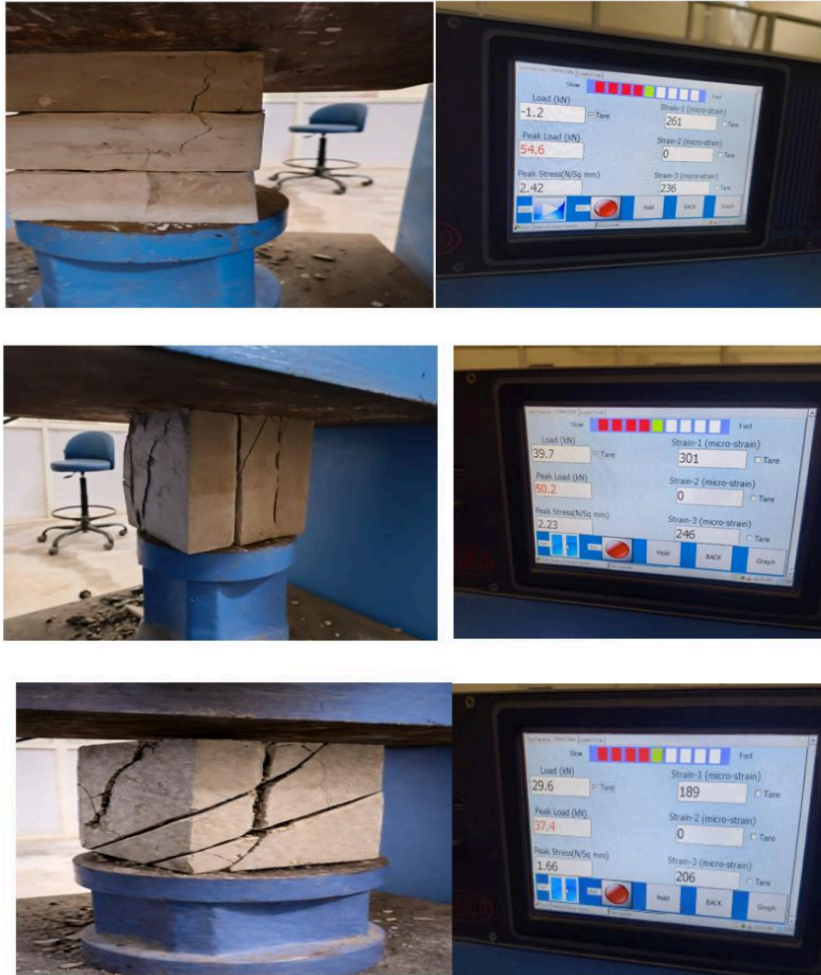
Figure 3.12 failure plane with no infill material
