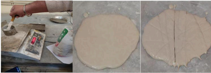
Figure 3.2 testing of setting time of gypsum plaster
