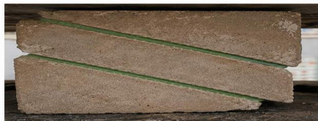
Figure 3.11 Arrangement of blocks with 30 degree orientation and 4mm infill material
