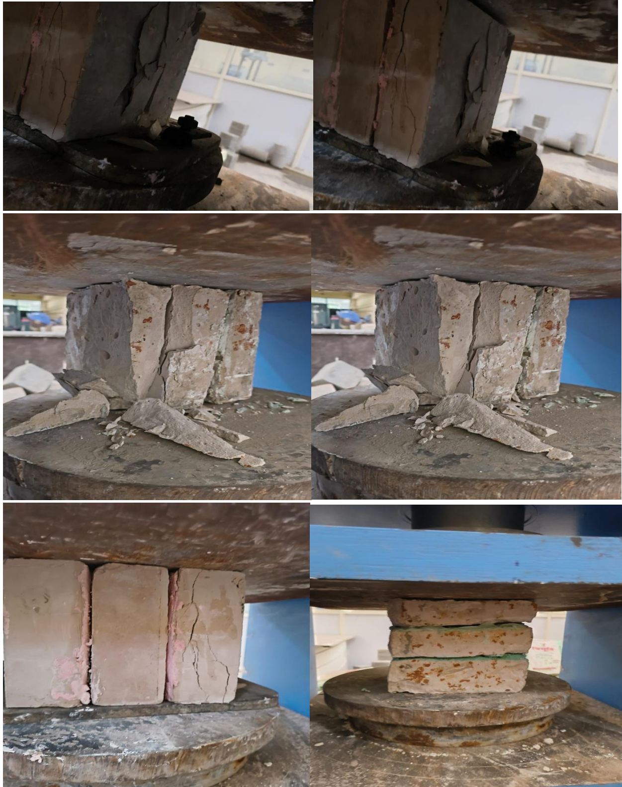
Figure 3.13 failure of blocks with 2 mm and 4 mm infill material
