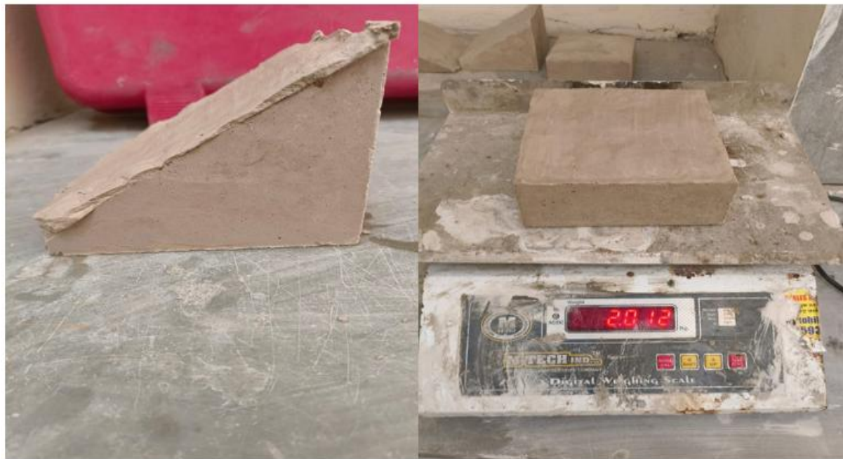
Figure 3.3 curing and weighing of blocks
