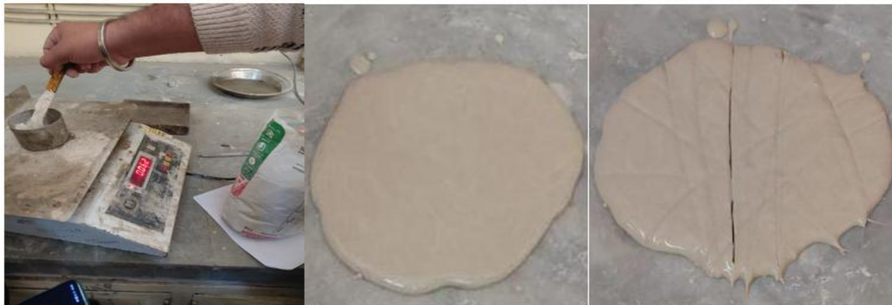
Figure 3.2 testing of setting time of gypsum plaster
