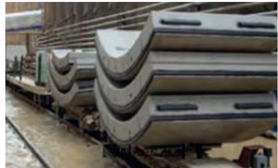
Fig. Segment Stacking for Storage & Transportation
