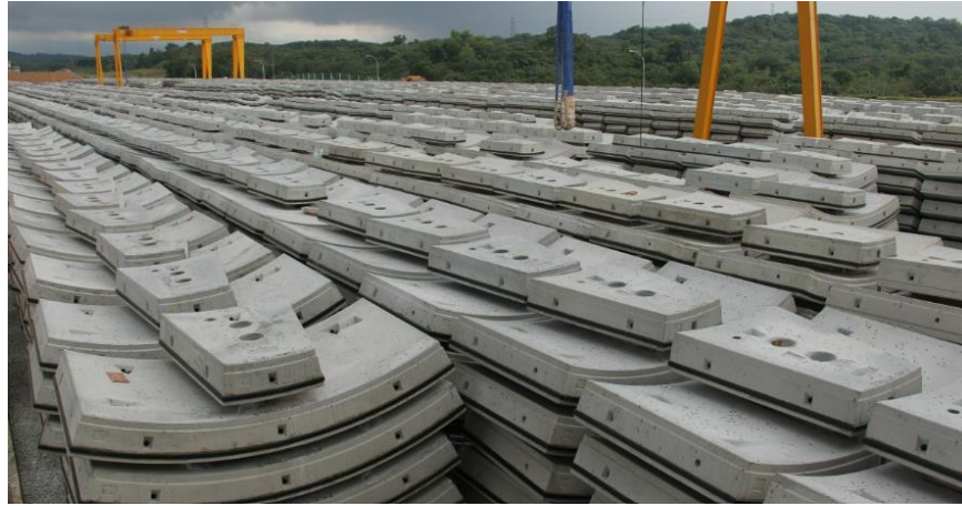
Figure 1.2: Photograph of Stacking of Precast Segments (Courtesy SPC Industries)
