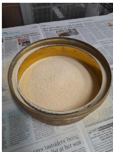
Fig. 6: Sample sieved using 850 \mu\text{m} mesh and stored in a cool and dry place for further use.
