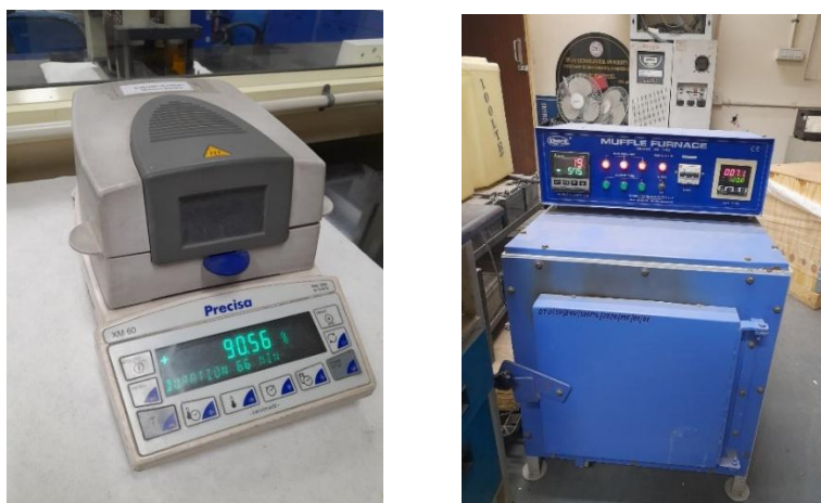
Fig. 7: Proximate analysis performed using Moisture Balance and Muffle Furnace from Water Engineering Lab and Solid Waste Lab respectively in Delhi Technological University.
