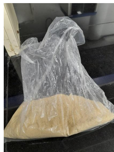
Fig. 6: Sample sieved using 850 \mu\text{m} mesh and stored in a cool and dry place for further use.
