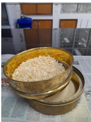
Fig. 6: Sample sieved using 850 \mu\text{m} mesh and stored in a cool and dry place for further use.
