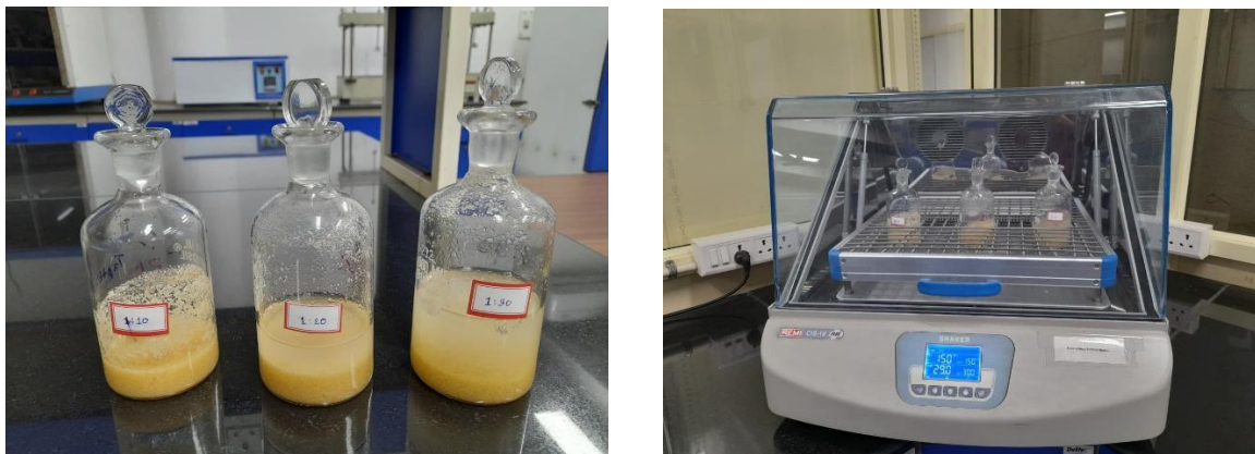
Fig. 13: Batch adsorption carried out using BOD bottles and orbital shaker.
