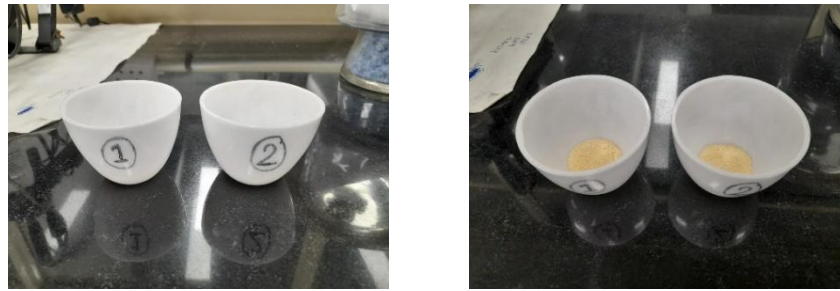
Fig. 8: Proximate analysis crucibles used to perform Ash and Volatile matter content in a Muffle Furnace.
