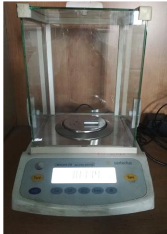
Fig. 3.4 Measurement of sample weight using an electronic weighing machine
