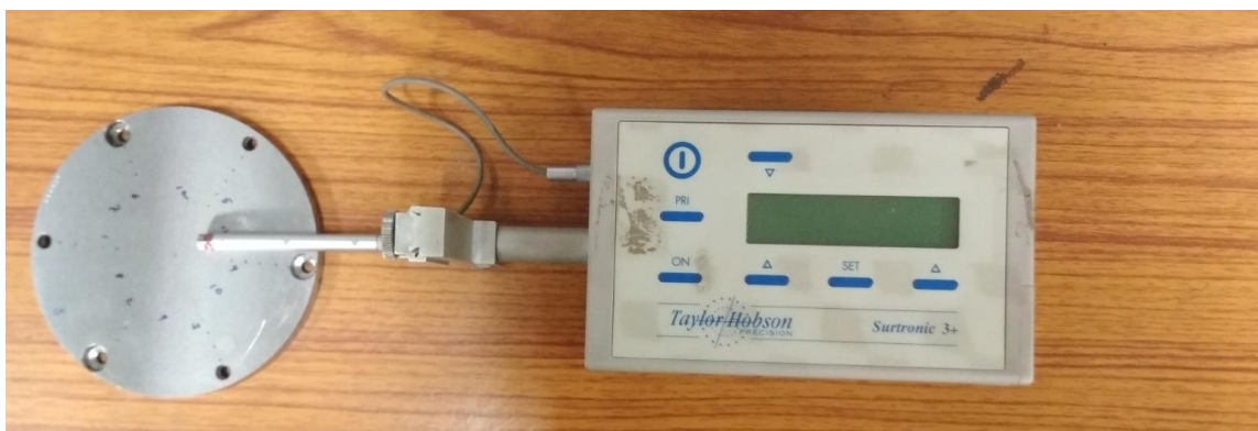
Fig. 3.3: Surface roughness checking on stylus surface roughness tester
