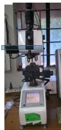
Fig. 3.1: Measurement of Vicker Hardness
