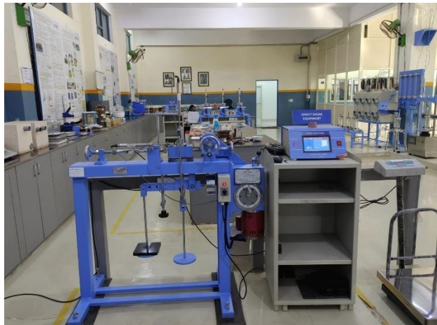
Figure 4.2 Arrangement of equipment for conducting the Direct Shear Test
