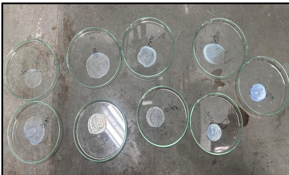
Figure 11: Gravimetric Method used for the determination of Solid Content and monomer conversion
