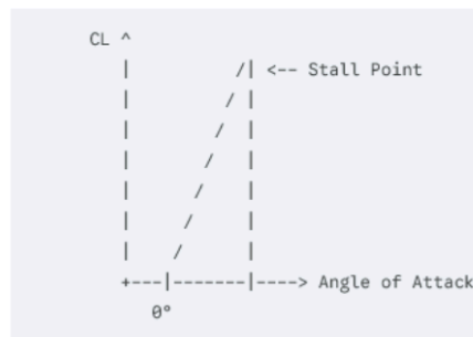
Figure 5: Typical lift coefficient (CL) versus angle of attack ( \alpha ) curve
