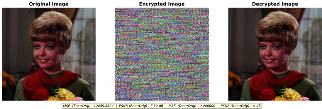
Figure 3.15: Original image (left), encrypted image (centre), and decrypted image (right). The encrypted image is visually indistinguishable from random noise. Decryption with the correct key recovers the original exactly: \text{MSE}(\text{Dec} \leftrightarrow \text{Orig}) = 0 , \text{PSNR}(\text{Dec} \leftrightarrow \text{Orig}) = \infty dB.
