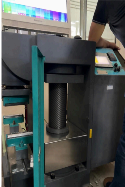
Figure 4.5: CFRP wrapped concrete cylinder under compressive strength testing
