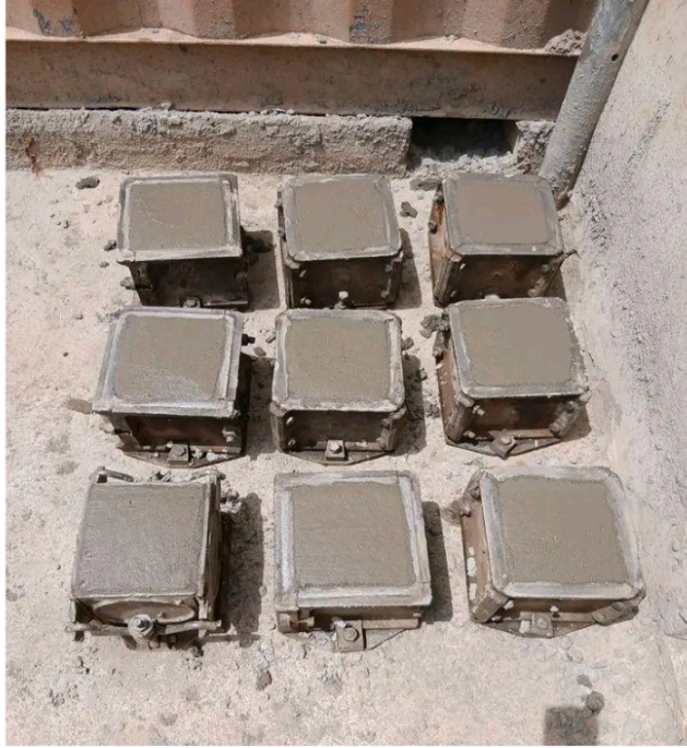
Figure 3.1 Casting of Concrete Cube specimens
