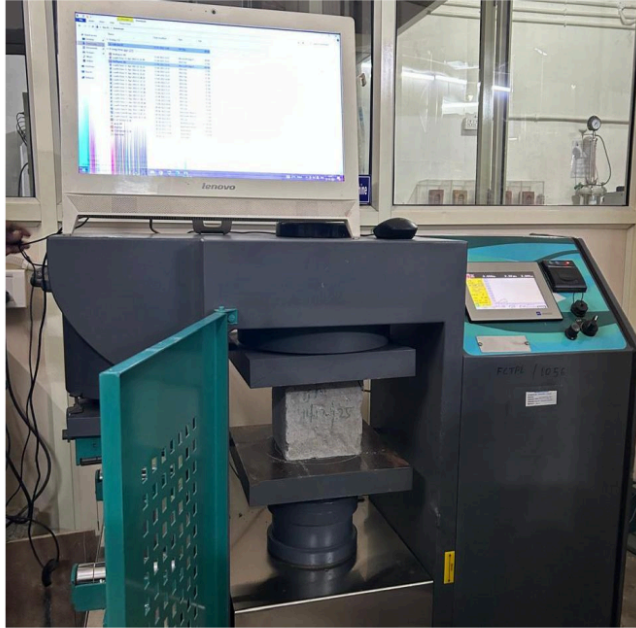
Figure 3.2: Compressive strength test setup for concrete cube
