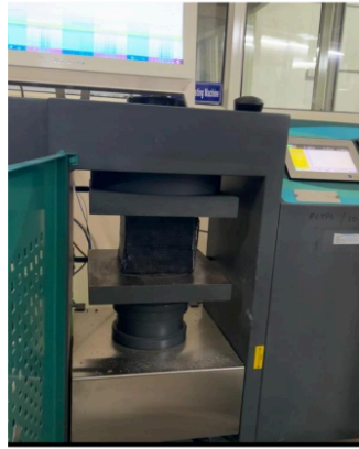
Figure 4.2: CFRP wrapped concrete cube under compressive strength testing
