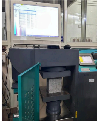
Figure 4.1: Concrete cube under compressive strength testing
