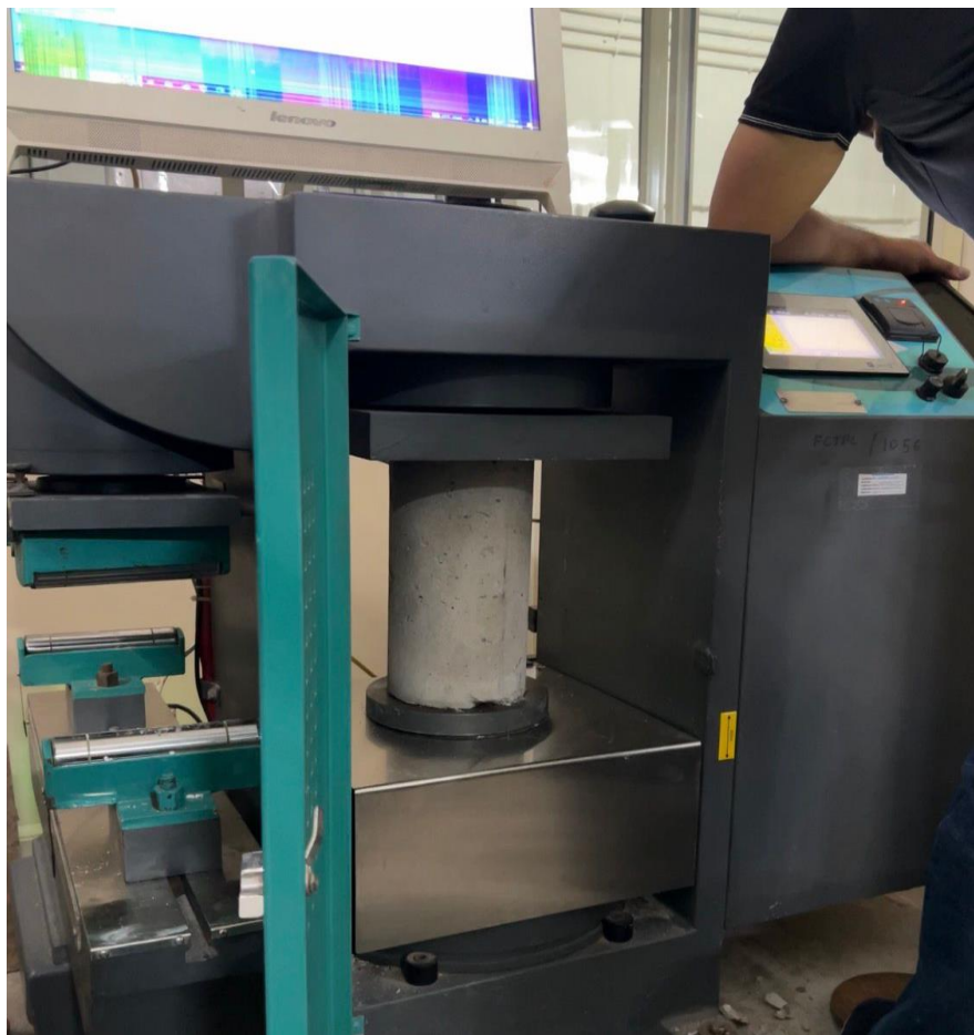
Figure 4.4: Concrete cube under compressive strength testing
