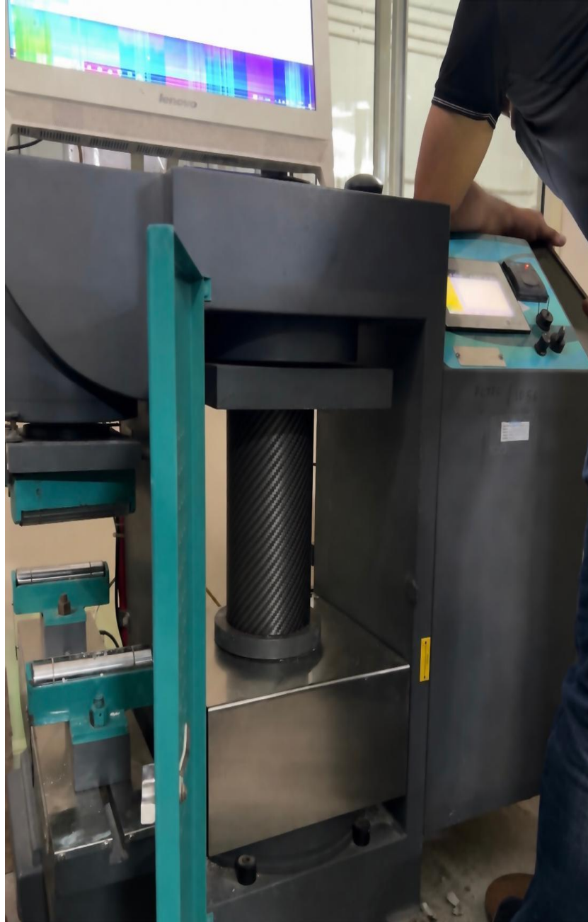
Figure 4.5: CFRP wrapped concrete cylinder under compressive strength testing
