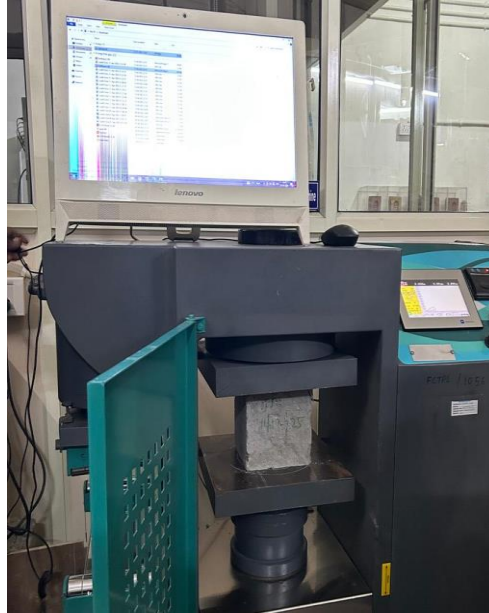
Figure 4.1: Concrete cube under compressive strength testing
