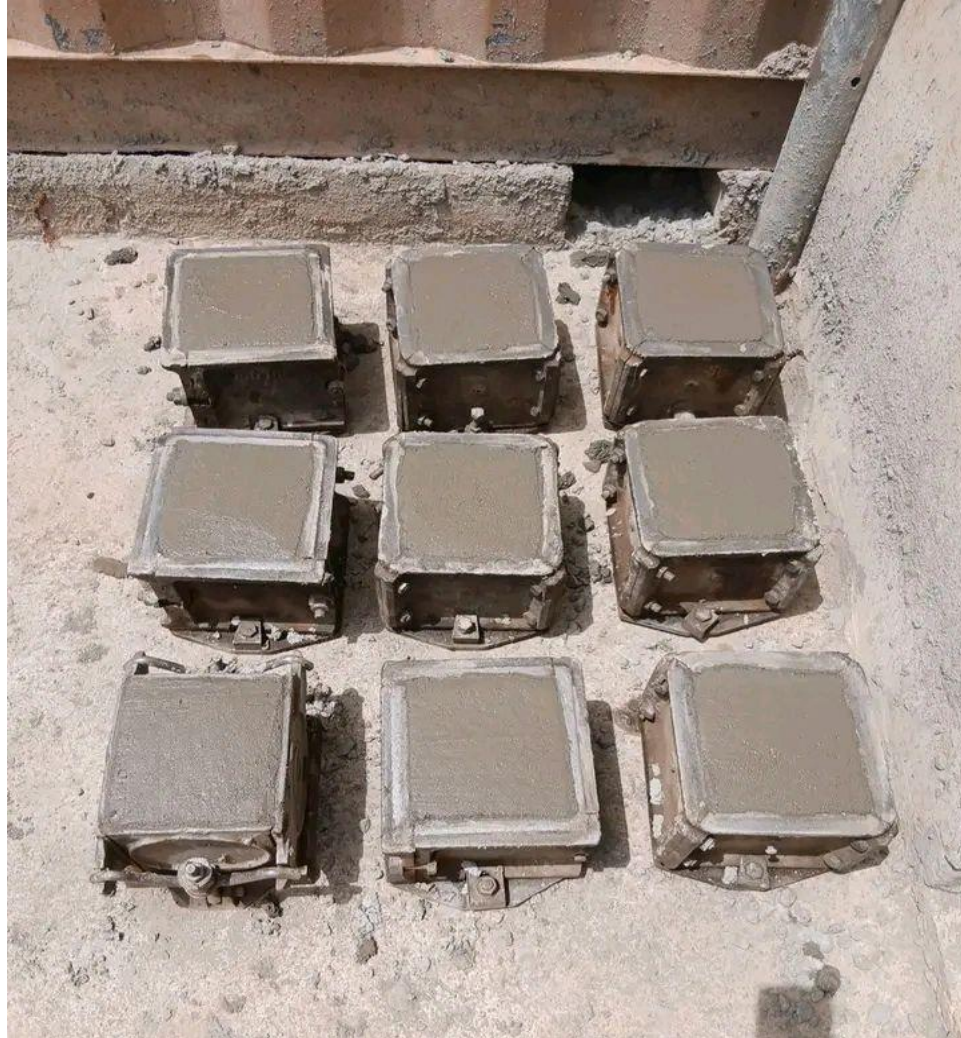
Figure 3.1 Casting of Concrete Cube specimens
