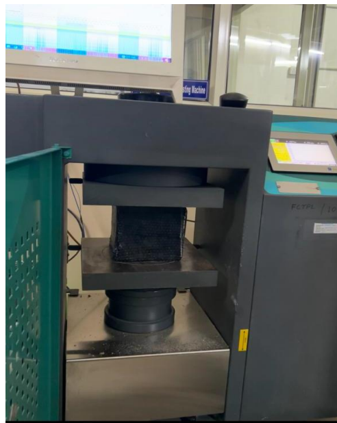
Figure 4.2: CFRP wrapped concrete cube under compressive strength testing
