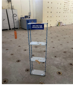
Figure 3.2: 3 Storey steel frame
