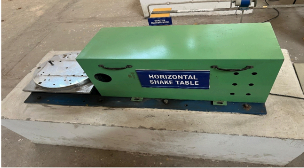
Figure 3.3: Horizontal Shake Table
