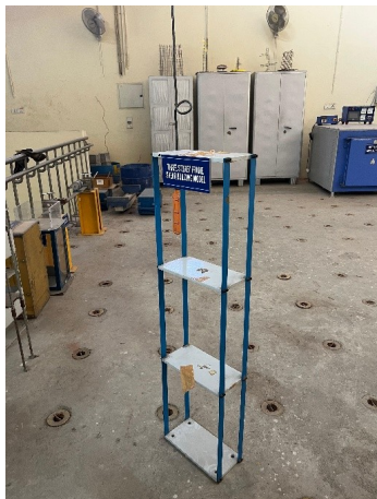
Figure 3.1: 3 Storey steel frame
