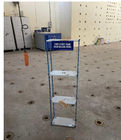
Figure 3.2: 3 Storey steel frame
