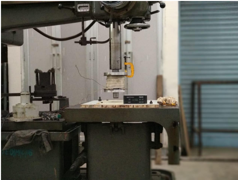
Fig. 32 Assembly of the electromagnet on the radial drill
