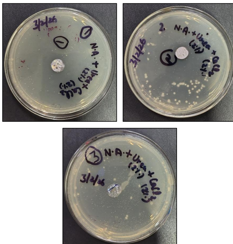
Figure 4.2: Comparative growth of bacterial isolates under optimum urea (2%) and calcium chloride (2%) concentrations.
