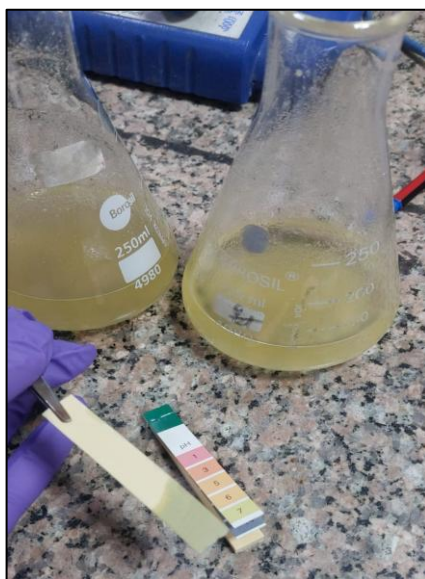
Figure 3.9: Experimental setup for evaluation of bacterial growth under alkaline pH conditions.
