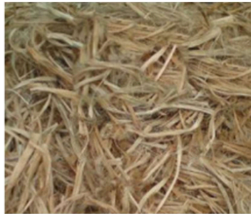
Figure 15: 45mm Jute fibre
