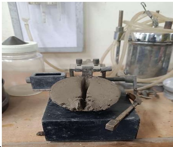
Figure 7: Liquid Limit Apparatus
