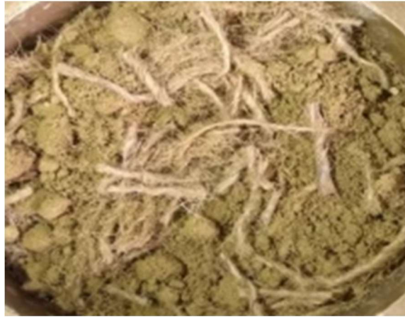
Figure 16 :Jute Fibre mixed in Soil Sample
