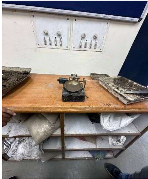
Figure 4.4: Casagrande apparatus used for evaluation of Atterberg limits
