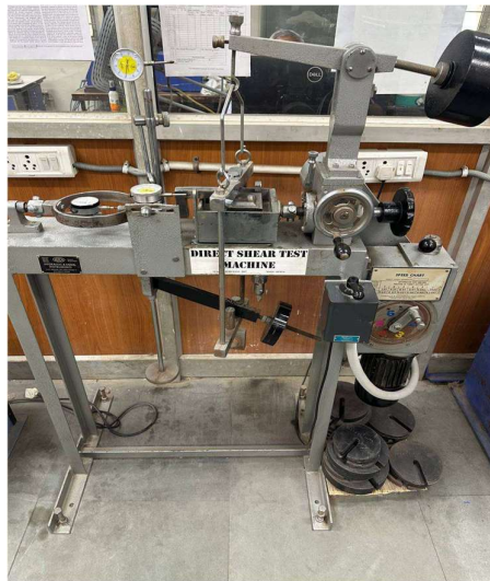
Figure 4.8: Apparatus used for determination of shear strength parameters
