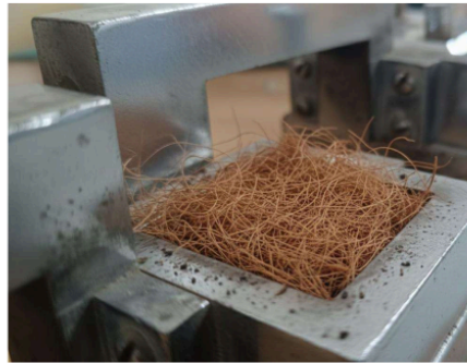
Figure 19: Reinforced soil sample
