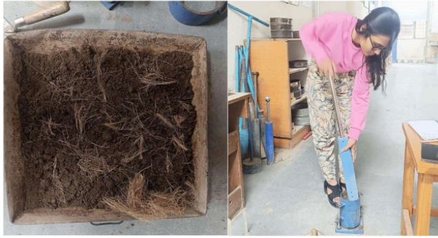
Figure 17: (a) 30mm coir reinforced soil (b) Compaction of coir fibres and dry soil
