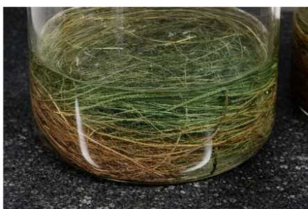
Figure 14: Pre-treatment of coir Fibres with \text{CuSO}_4
