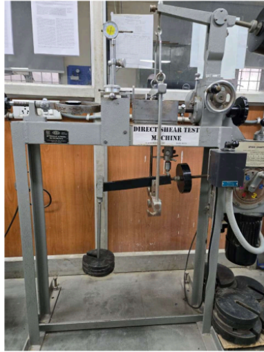
Figure 18: Direct Shear testing machine
