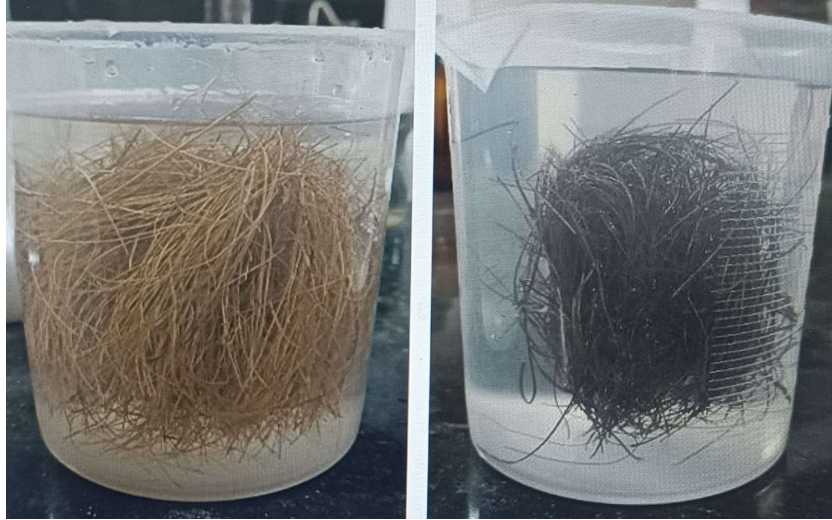
Figure 16: Water absorption test on a) Untreated coir Fibres & b) CNSL-treated coir Fibres
