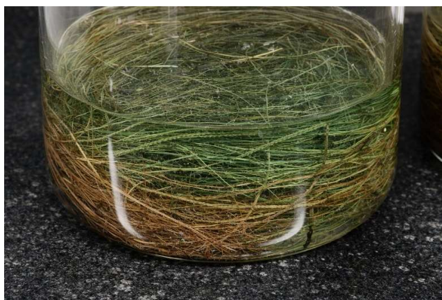
Figure 14: Pre-treatment of coir Fibres with \text{CuSO}_4
