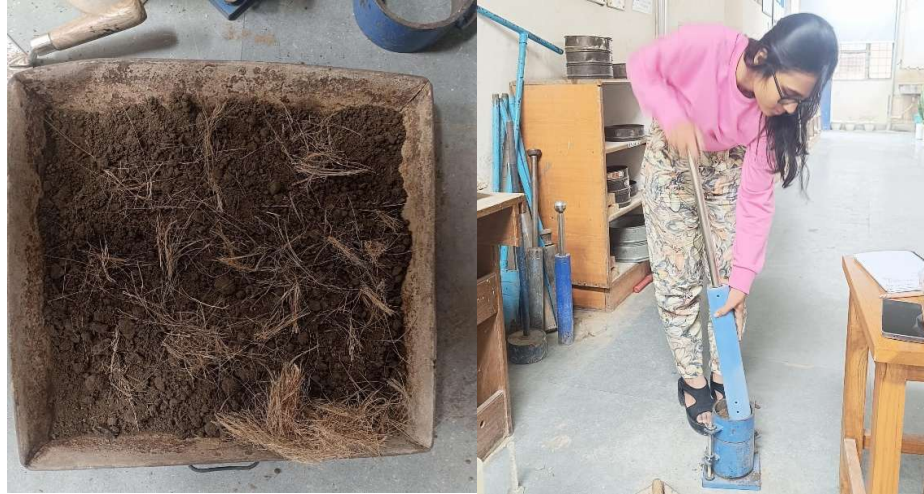
Figure 17: (a) 30mm coir reinforced soil (b) Compaction of coir fibres and dry soil
