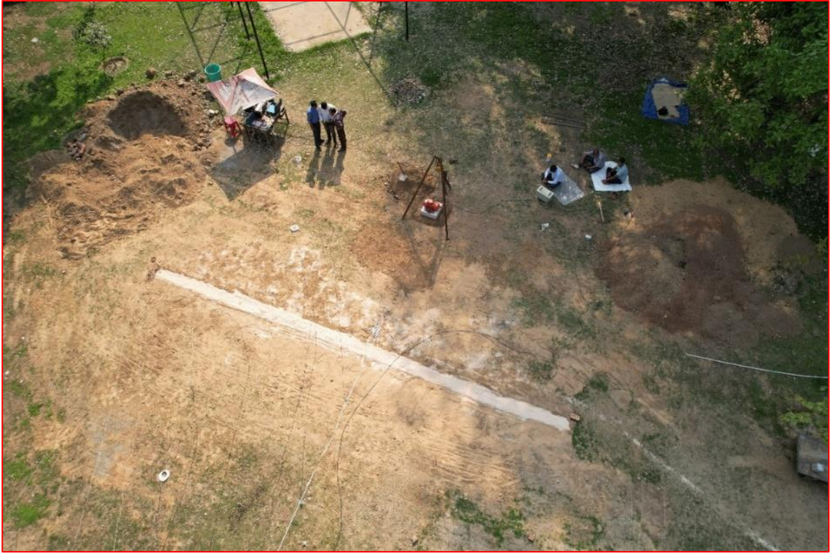
Figure 35: Aerial view of In-filled trench wave barrier
