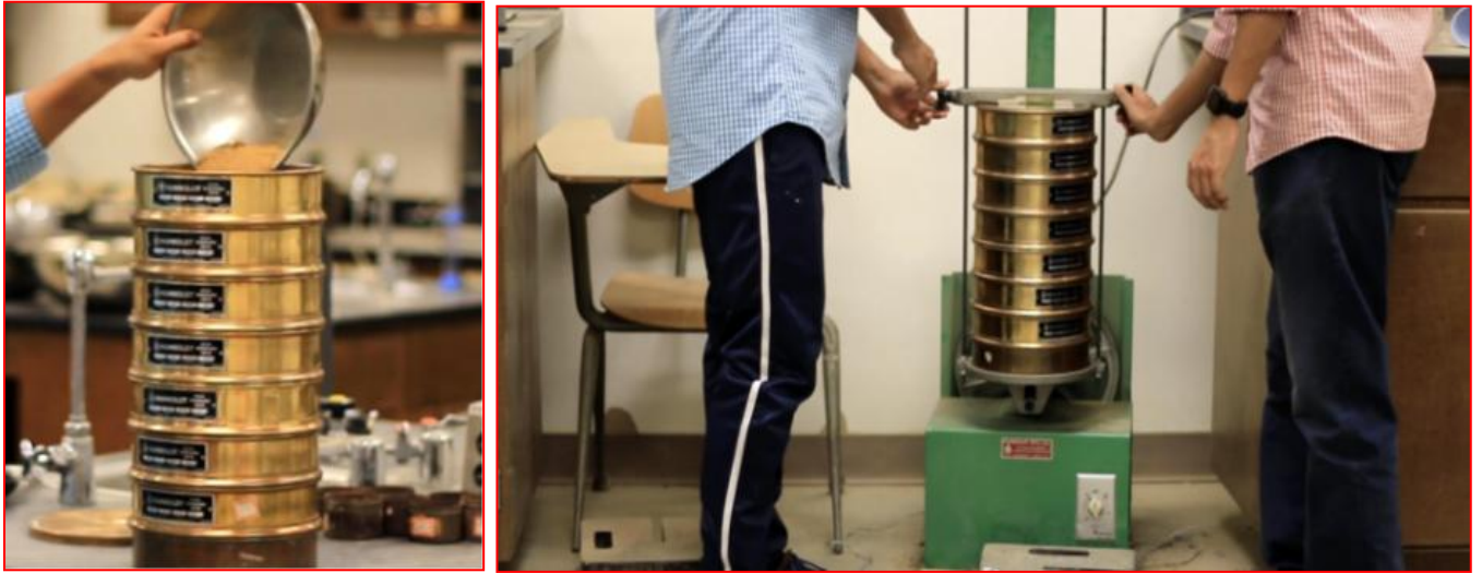
Figure 19: Pouring the soil sample on sieves and vibrating on sieve shaker
