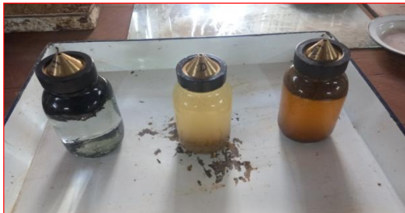
Figure 21: Testing for Specific Gravity of the in-filled materials
