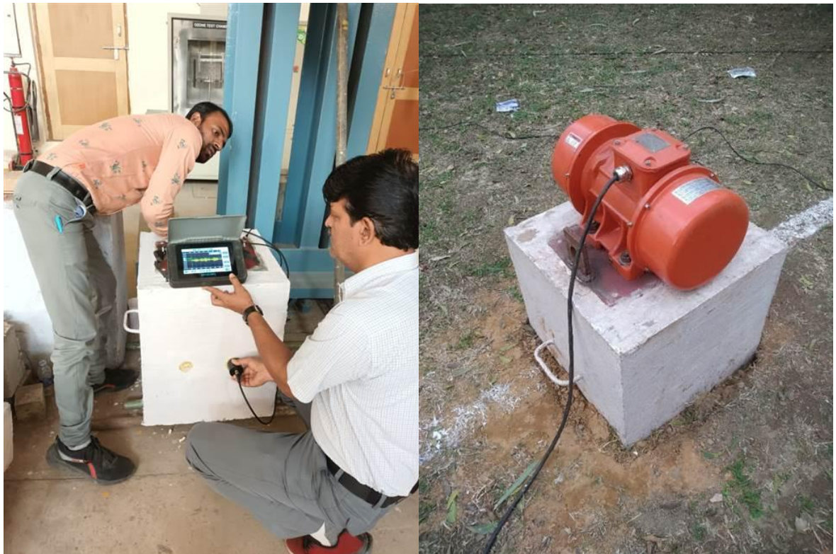
Figure 72: View of Electro-Mechanical Oscillator & Testing of its Footing
