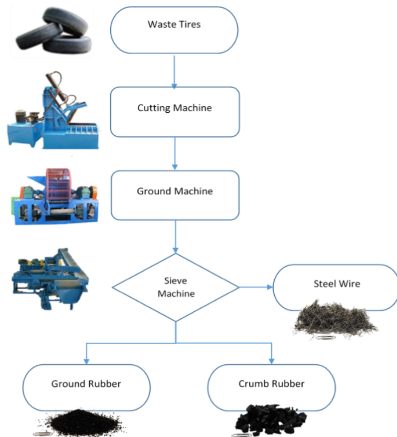
Figure 16: Layout of the process for formation of Crumbed Tyre Rubber from waste Tyres (Source: Journal of Engineering Science and Technology, No. 1(2021) 510-526), Volume-16
