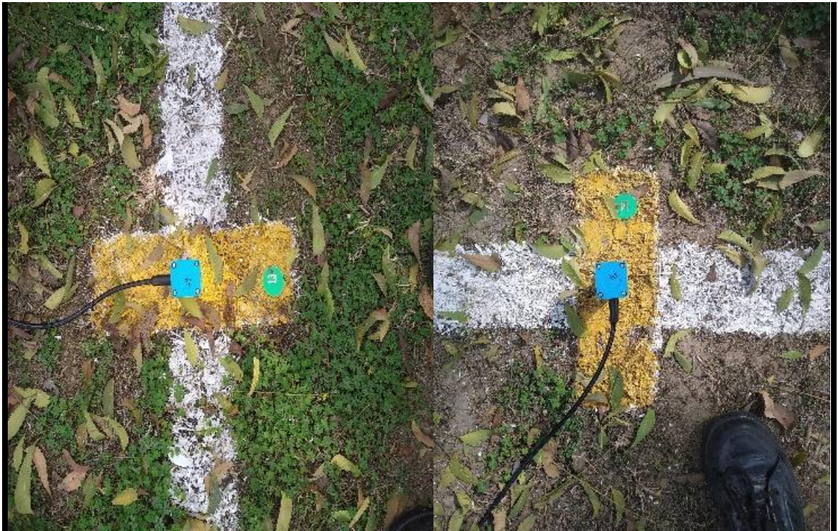
Figure 73: Installed Geophones on the centre line of the profile
