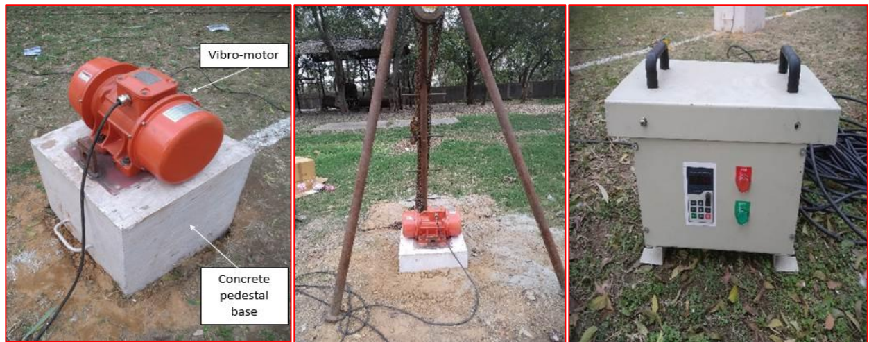
Figure 31: View of Electro-Mechanical oscillator, tripod and Variable Frequency Drive (VFD)
