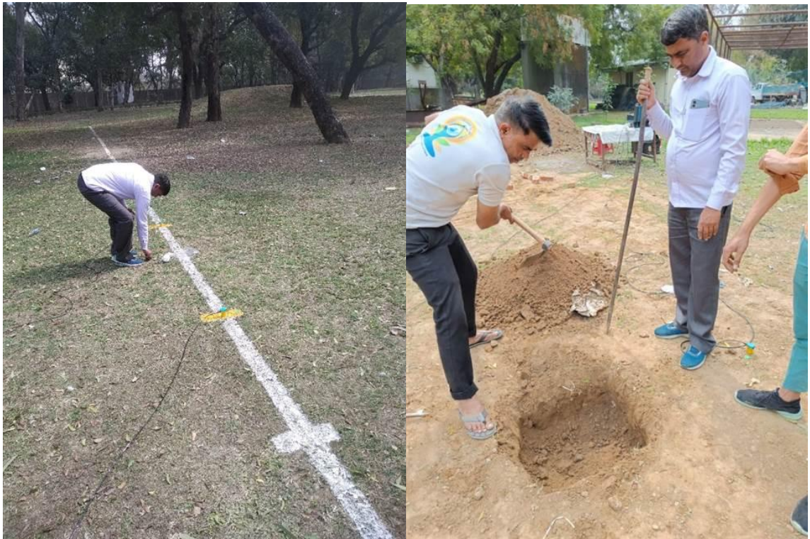
Figure 67: Installation of Geophones and excavating pit for Oscillator
