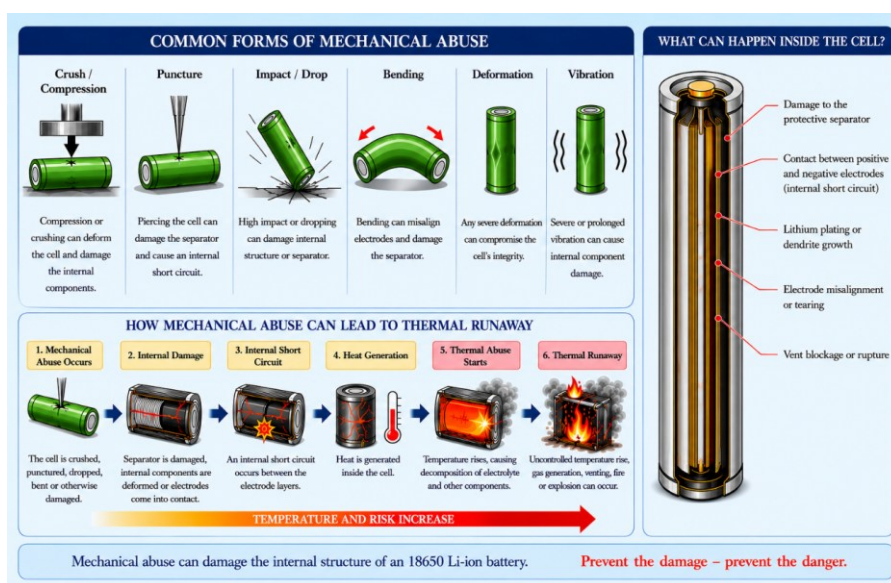
Fig. 3.5 Schematic Illustration of the Mechanical Abuse
