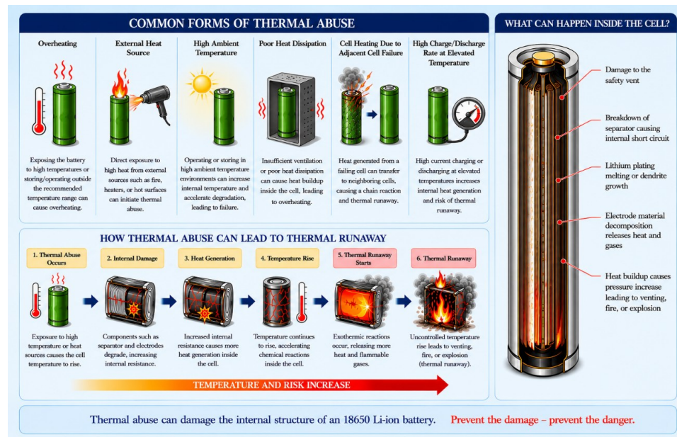
Fig. 3.4 Schematic Illustration of the Thermal Abuse
