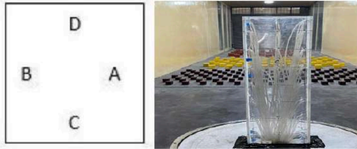
Fig.5.1: Plan and fabricated model of square structure
