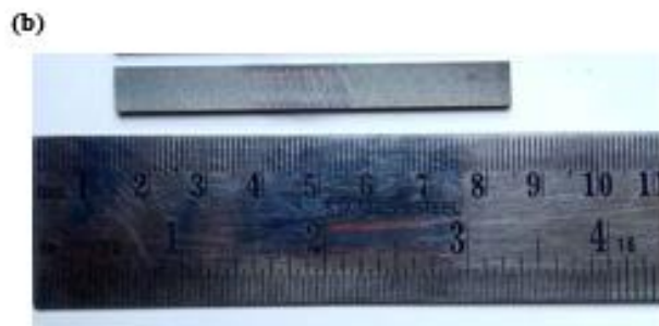
Figure 3.10 (a) Schematic diagram of 3-point bending test specimen b) Prepared samples along with scale c) Bending Specimen
