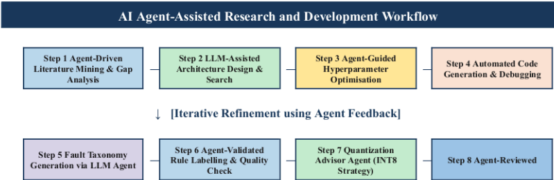
Figure 3.9: Development Pipeline of Eight Steps From Literature Mining to Architecture Design, Hyperparameters Tuning, Fault Labeling, INT8 Quantization Strategy, and Review
