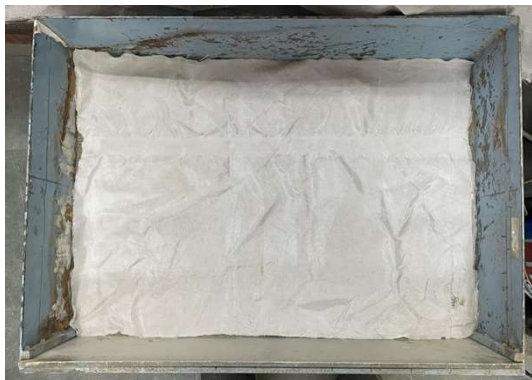
Fig. 5.12 shows geosynthetic in test tank
