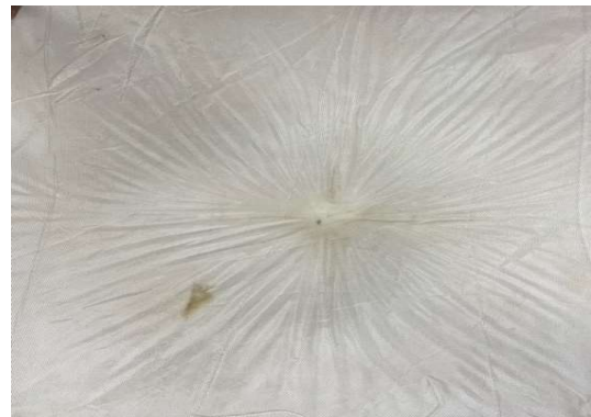
Fig. 5.13 shows geosynthetic after DCPT
