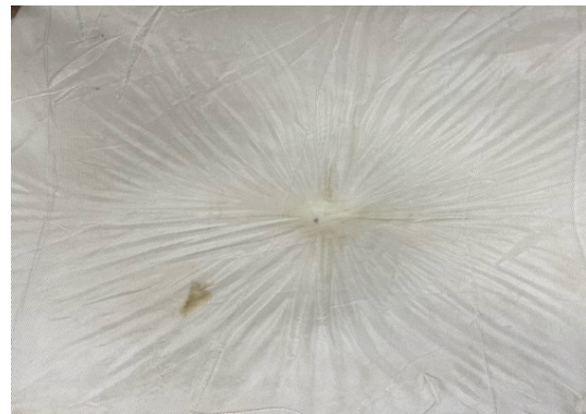
Fig. 5.13 shows geosynthetic after DCPT
