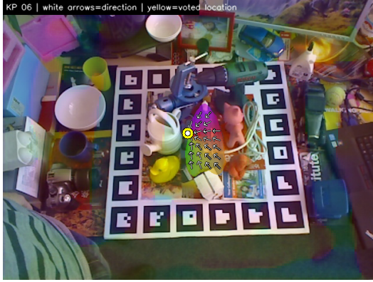
Figure 4.2. Predicted unit vector field for keypoint 6. White arrows show the per-pixel direction predictions; the yellow dot marks the voted keypoint location.
