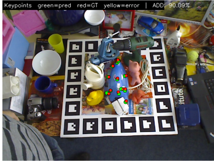
Figure 5.4. Predicted keypoints (green) versus ground-truth keypoints (red) on the iron object. Yellow lines indicate the per-keypoint error. The ADD accuracy for this frame is 90.09%, demonstrating close alignment between the voted keypoint locations and the ground truth.
