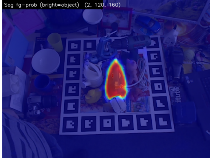
Figure 5.3. Predicted segmentation probability map for the iron object, overlaid on the RGB input. Bright regions indicate high foreground probability. The segmentation cleanly isolates the target object from the cluttered background.
