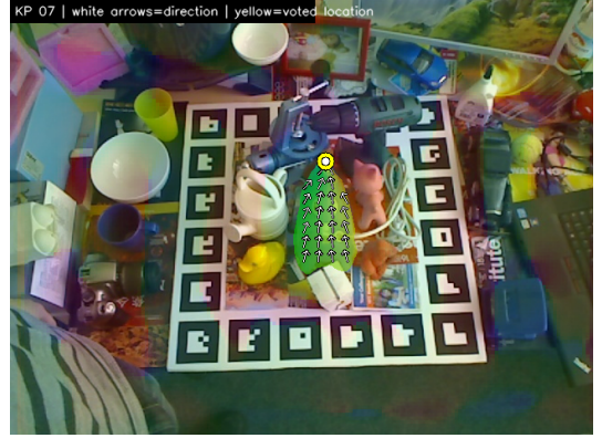
Figure 4.3. Predicted unit vector field for keypoint 7. The arrows converge coherently toward the voted location, demonstrating that the network has learned geometrically meaningful direction predictions.
