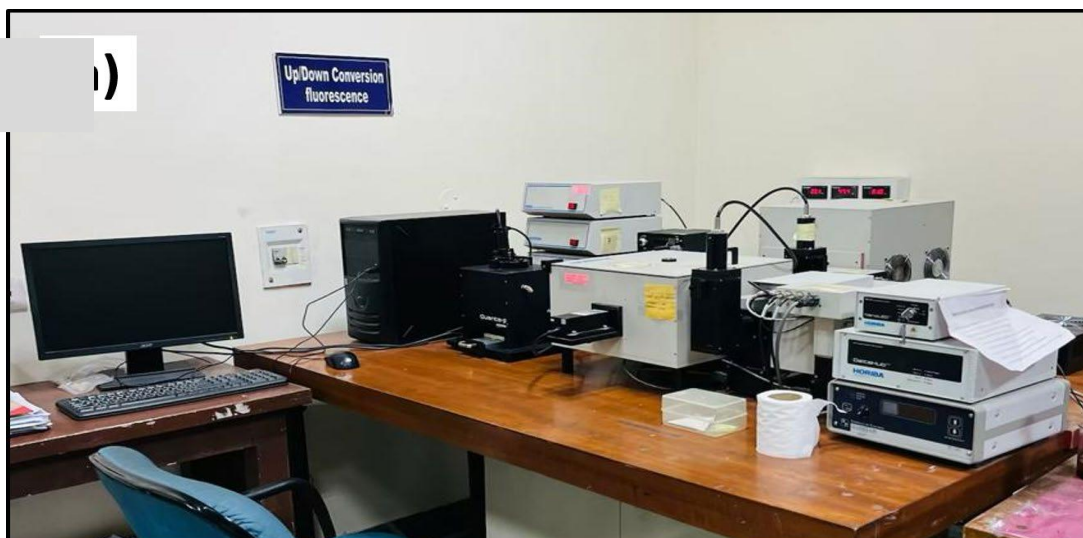
Fig. 2.9. Upconversion luminescence measurement setup using a Horiba PTI QuantaMaster spectrofluorometer with a 980 nm laser.
