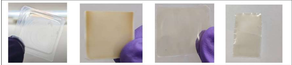
Figure 3.2: Photograph of synthesized nanocomposite films (a) PVDF. (b) Bi 2 O 3 /PVDF. (c) Au-NPs/PVDF. (d) Au-NPs/Bi 2 O 3 /PVDF.
