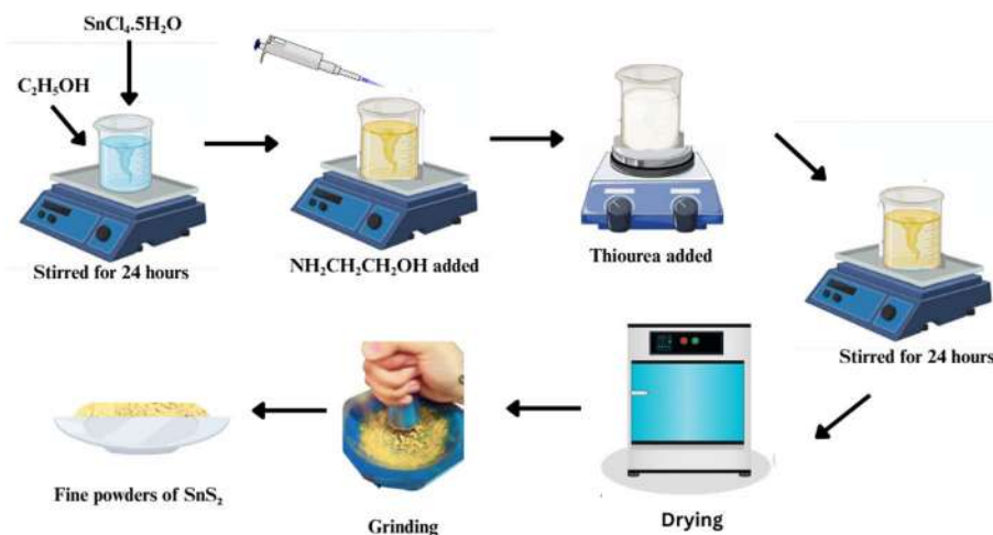
Fig. 1 Schematic diagram of the process involved in the synthesis of SnS 2 nanosheets
