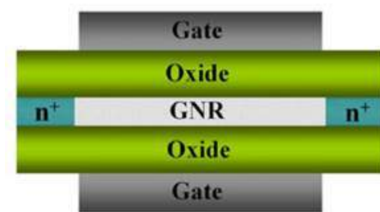
Figure 1.15: MOS type GNRFET with doped source and drain extensions [43]
