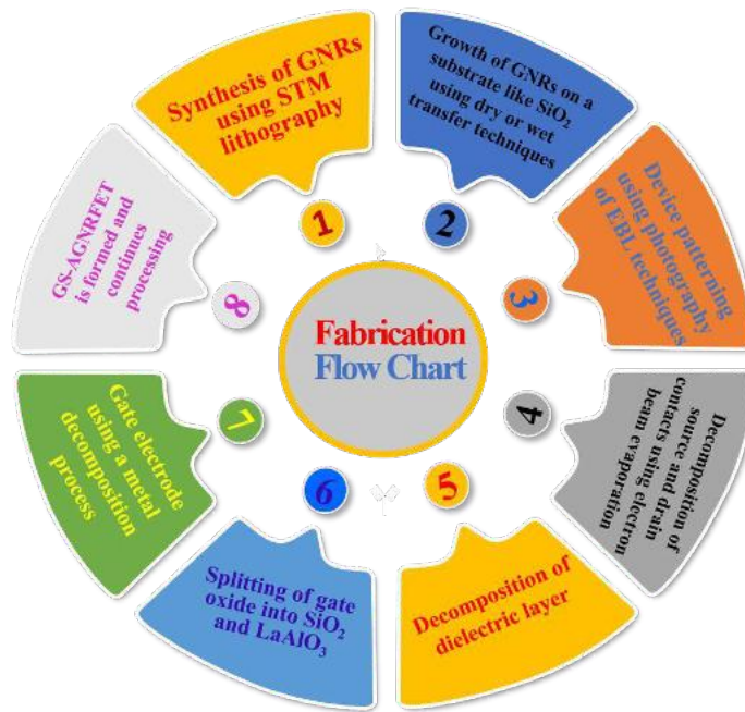
Figure 2.4: Fabrication flow chart for GS AGNRFET device [36]
