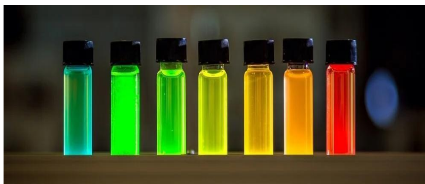
Figure 1.2: luminescence in different colour ranges on the basis of chemical composition, phosphors can be categorized into organic and inorganic phosphors.
